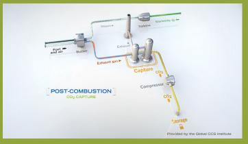
**Post-combustion** processes separate CO2 from combustion exhaust gases. CO2 can be captured using a liquid solvent or other separation methods. In an absorption-based approach, once absorbed by the solvent, the CO2 is released by heating to form a high purity CO2 stream.
